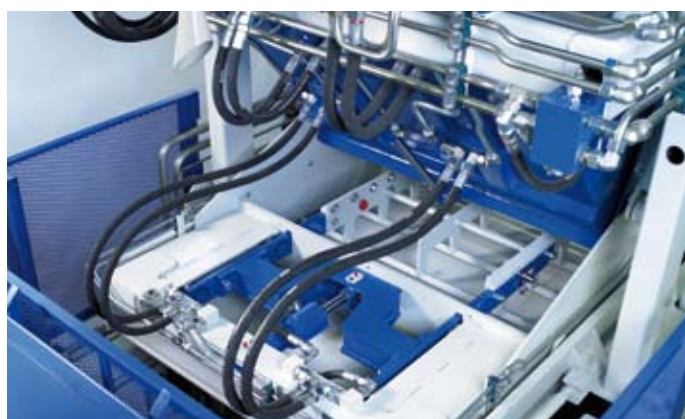
Fig. 1 Hydraulically driven grate for feed drawer
