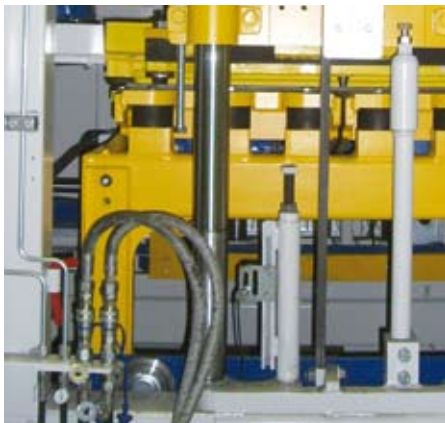
Additional connection capabilities for special moulds hydraulically driven
