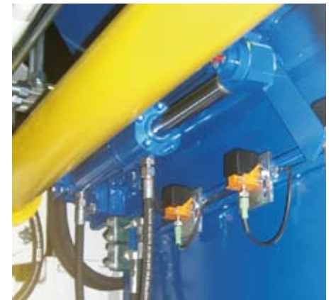
Hydraulic drive for turning flap
