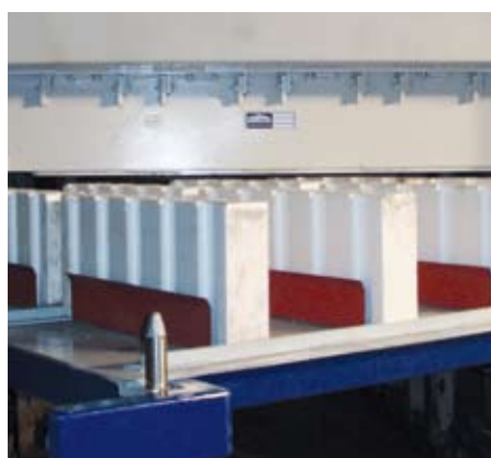
Fig 3 Device for insertion of polystyrene cores
