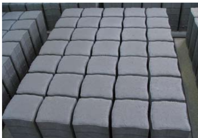
Fig. 2: Paving blocks manufactured on the Zenith 844 multilayer machine.
