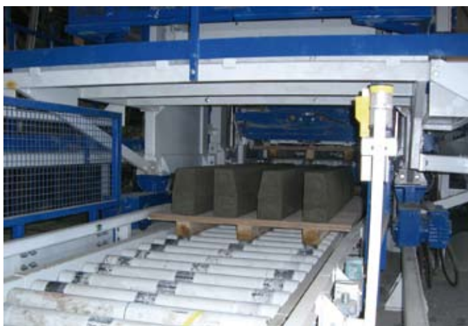
Fig. 1: Curbstone production with the Zenith 844 on the pallet roller conveyor.
