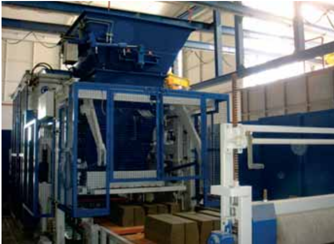
The HB 865 blockmaker is equipped with a special silo for facing concrete, thus enabling the production of multicoloured elements
