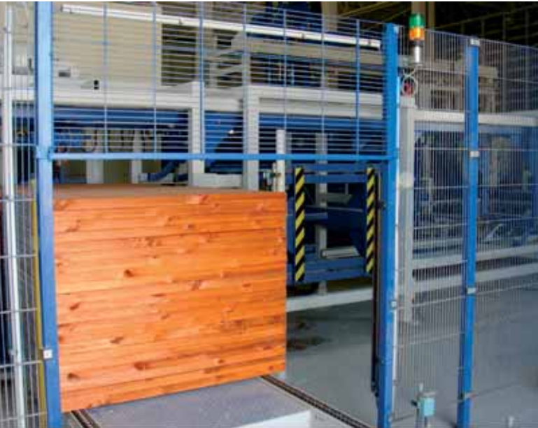
Board return transport system with an intermediate storage space for inserting and removing surplus manufacturing boards
